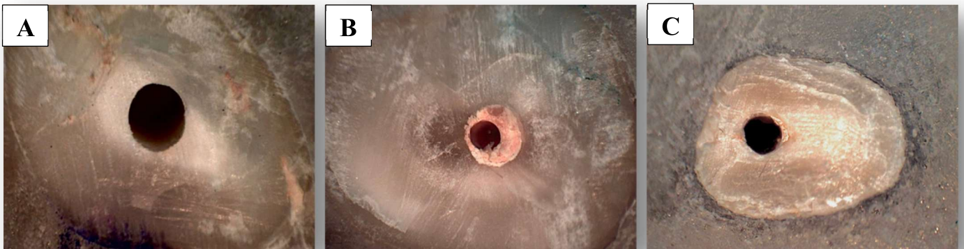
Figure (4.9): Stereomicroscope view mode of failures: (A) Adhesive failure, (B) Cohesive failure, (C) Mixed failure
