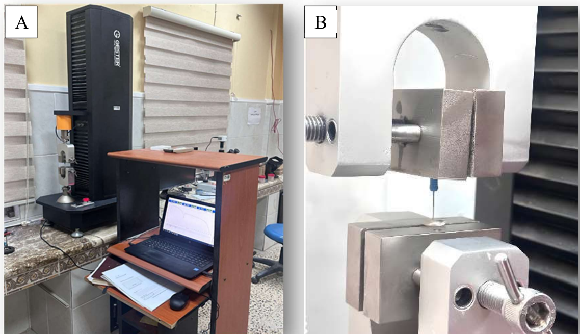
Figure (3.21): (A) Universal testing machine, (B) The sample centered under the plunger with metal base
