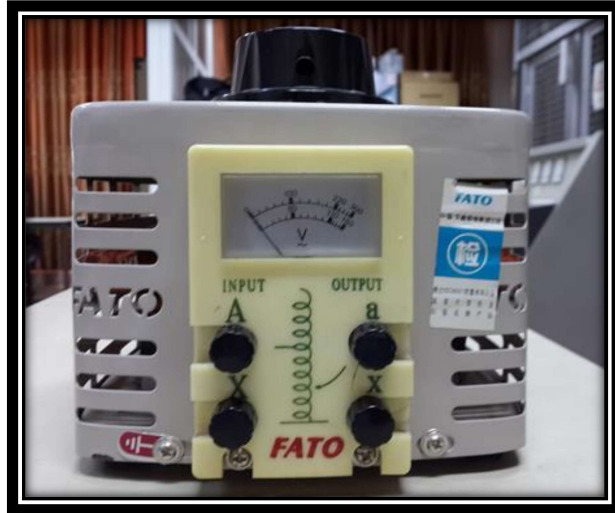
الشكل (13-3) : (auto transformer)
